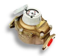
The V300 is a highly accurate volumetric rotary piston type meter used for the measurement of drinking water. Its specially developed thermoplastic measuring chamber assembly is extremely resistant to aggressive water and provides a long working life. The meter starts to register at very low flows and is accurate throughout a wide flow range.
