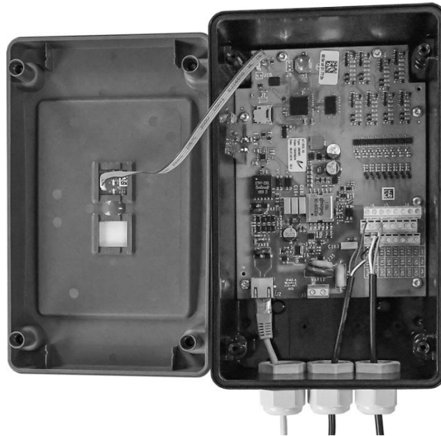
Figure 2: Inside of the iDOL 63 box. Make sure that cables and wires are connected as illustrated
