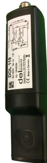
DOL 119 is a sensor for measuring carbon dioxide/CO2. The sensor is intended for measurement in live-stock houses and industrial environments.
