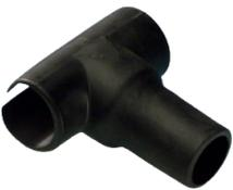
The T-bracket makes it easy to mount 30 mm sensors on plastic pipes in pipe systems where the sensor detects the material through the plastic wall of the pipe. The bracket is suitable for pipes with diameters between 40 and 60 mm.
